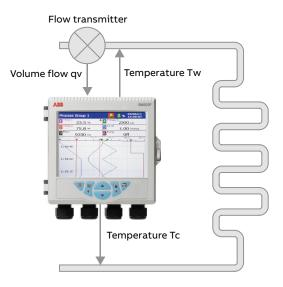
Temperature Tw is the temperature of the water in the supply side of the system. This is the water entering the chiller unit and providing the chilling function for the cold air. Temperature Tc is the temperature of the water in the return side of the system; this is the water that has been used to cool the air and is now at a higher temperature. Finally, qv is the flow of water through the system at the supply side.
